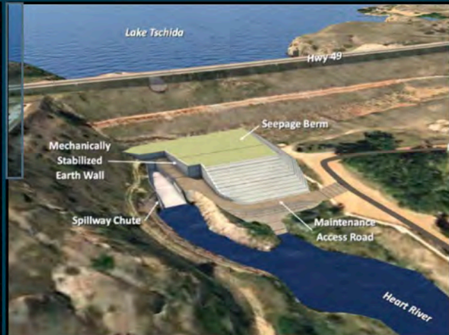
View of planned seepage berm
