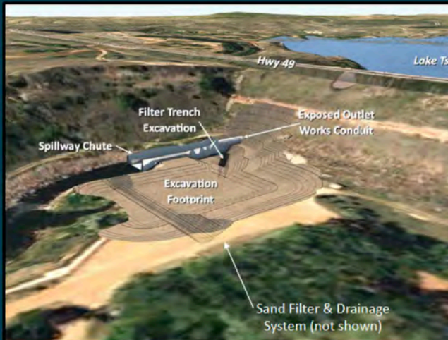
Planned excavation for filter installation
